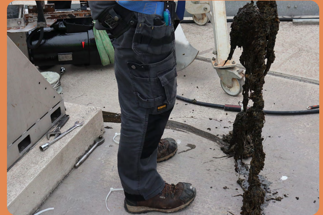
FIGURE 8: 'ROPES' OF UNDEFINED COMPOSTABLE PLASTIC MERGING IN A MESOPHILIC WET DIGESTER TO FORM A FLOATING LAYER
