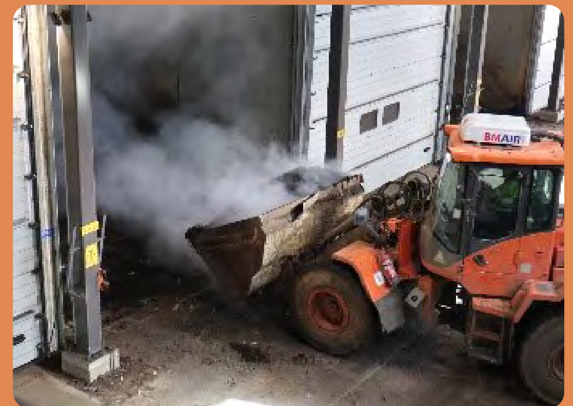
FIGURE 13: SOLID DIGESTATE IS MOVED TO NEXT PROCESSING STEP AT THE INTEGRATED IN-VESSEL COMPOSTING PLANT
