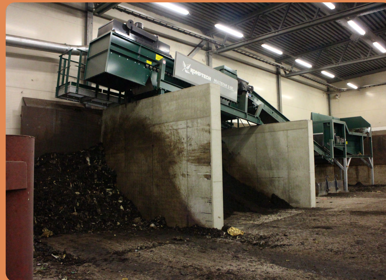
FIGURE 11: AFTER A RETENTION TIME OF 30-35 DAYS, DIGESTATE IS DEWATERED, COMPOSTED, THEN SCREENED.
