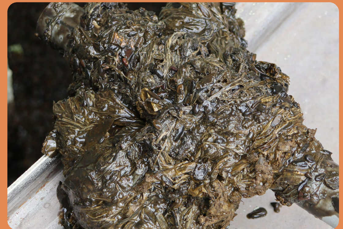
FIGURE 9: CLOSE UP OF COALESCED COMPOSTABLE PLASTIC FORMING A FLOATING LAYER IN A MESOPHILIC WET DIGESTER
